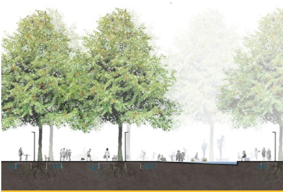
Redevelopment of a square with green spaces, water permeable surfaces, and water elements; square rainwater storage and capacity to reuse that rainwater in the square for irrigation; root protection elements in trees with perforated caps; and use of new technologies that create a root protection substrate.
